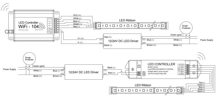
Actual wire colours may vary - follow labels on the units Recommended to add 10% buffer when sizing power supply LED drivers require enclosures
