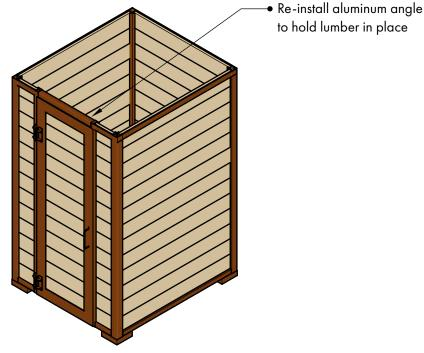
Position the roof and adjust the frame to line up all of the threads. Insert all fasteners loosely to ensure proper alignment before final
