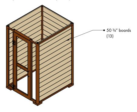
On the front, slide in the plastic lumber from the top in the same way with groove down, tongue up, and textured side out. Remove the aluminum angle and install the plastic lumber on the door last. Note decal board position.
