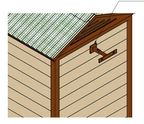
• Position connecting fixture and drill four 17/64'' holes through the plastic lumber on the back wall. Attach with SJ0614 ( $1/4'' \times 2 1/4''$ ) carriage bolts (4) from the inside and SB0505 (1/4'') flat washers and SA0605 (1/4'') hex nuts (4 of each) on the outside.
