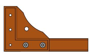
Stand the panels on edge with the channels facing each other as shown. Attach the flat bar side support to the top of the panels on one side of the frame.
